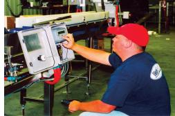
Our products feature our patented WeighTech indicator. Our permanently sealed MicroWeigh indicator complies with industry standards for protection from water ingress under IPX9K (pressure washing), NEMA 4 (hosedown), NEMA 6 (water immersion), IPX7 (water immersion) and IPX8 (water immersion simulating water pressure over 80-feet deep). MicroWeigh has also satisfied tests for dust resistance under IP6. We know of no other manufacturer of an electronic indicator that has passed all these tests.
